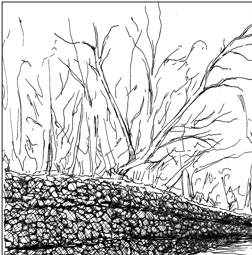
Figure 1. Gabion revetment on streambank
