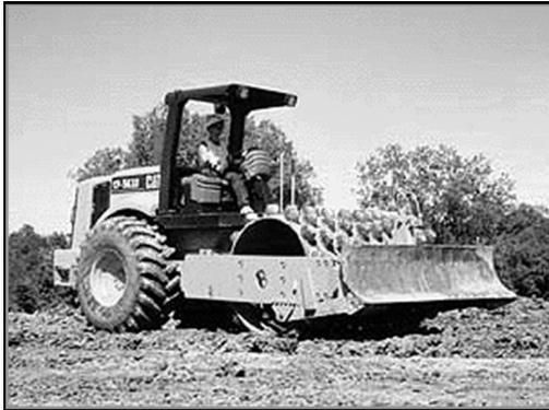
Sheepsfoot roller used for soil compaction
