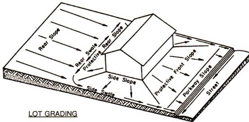
The picture above illustrates the most common drainage problem of a sloping lot. The uphill side of the house must have a drainage waterway (swale) to direct the water around the house. This drainage swale should be at least ten feet from the house and sloped to convey accumulated water away from the dwelling efficiently, and into a proper outlet.
